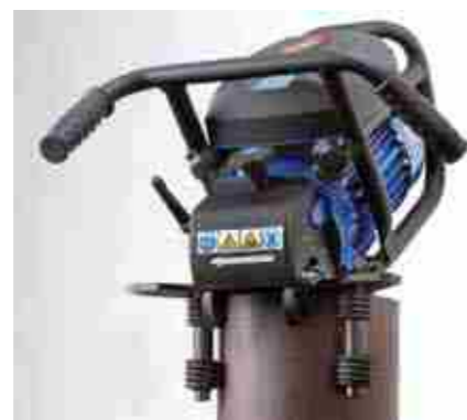
Edge machining on vertical pipes
